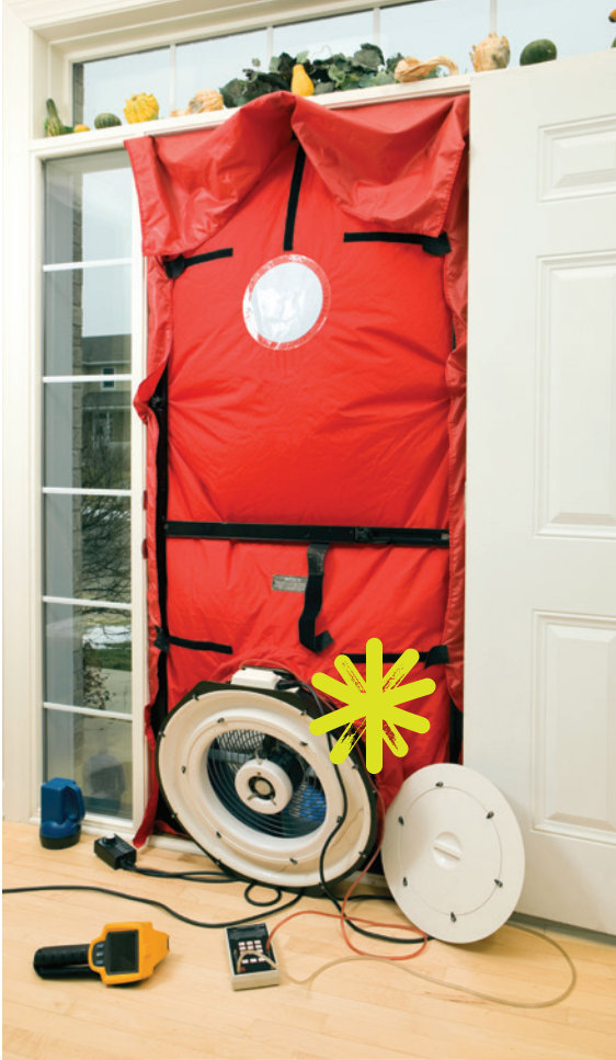
A blower door test can identify gaps in your home, large and small.
